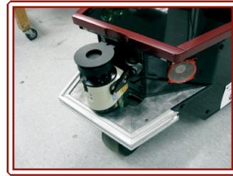
**Figure 3: LIDAR Mounting**
