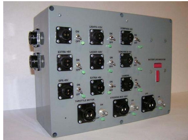
Figure 6: Warrior Power Distribution Box
